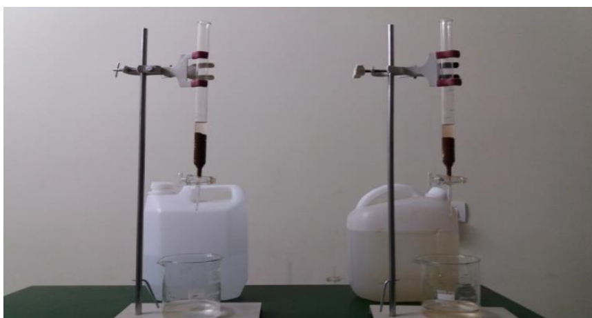
Fig 4. Column study for benzene removal
