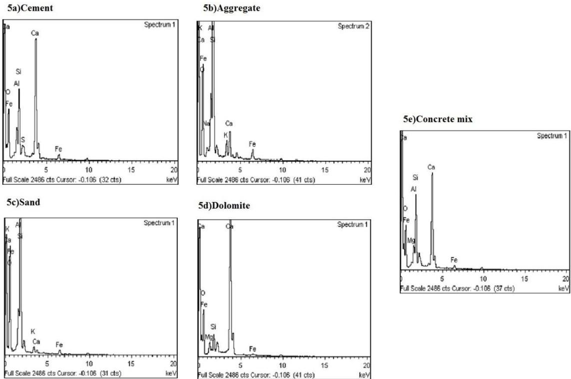
Energy dispersive X-ray (EDX) analysis is used for the determination of elemental composition and some of the specific elements in the adsorbent material, the figure. 5 and 6 of images shows that different peak positions and their elemental composition are Mg=1.93%,O=77.63%,Si=2.20%,Fe=0.26%.Ca=17.98%. After combination of cement and dolomite powder the concrete mixture the elemental composition also increased.
