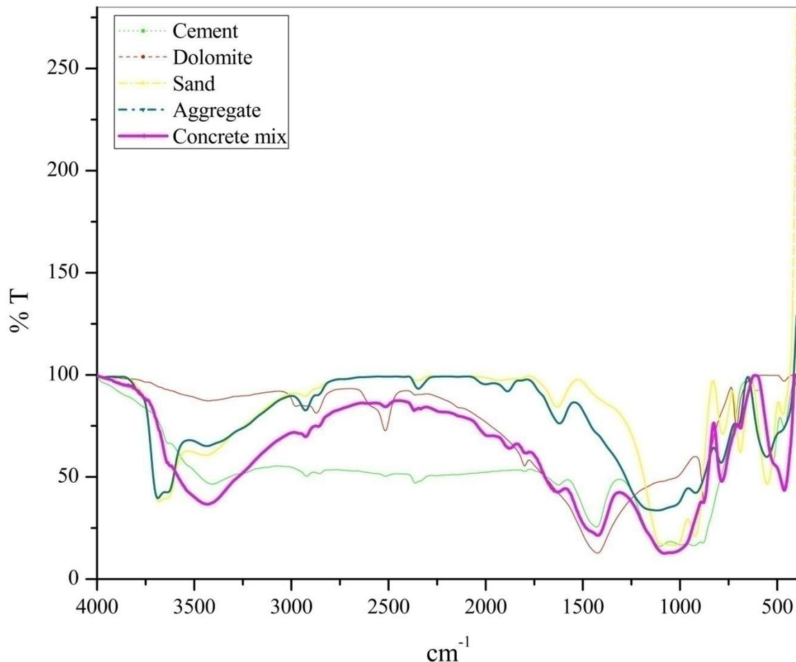
Fig. 4. FTIR Spectrum of cement composition: without additive and with dolomite additive.
