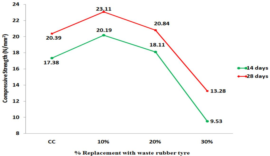
Fig. 2. Compressive strength in Water curing
